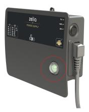
If an automatic cover dry contact is connected to the box, the switch present on the side of the box should be in EXT position to enable detection. It is still possible to flip the switch to 100% to disregard the tank cover information and force nominal production, or even to 25% to divide the production by 4 regardless of the status of the shutter.
