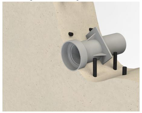
Then bond a seal before fitting the liner
