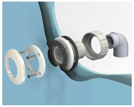
The connection at the back of the wall crossing is to a tube using a 1.5" threaded connector.
