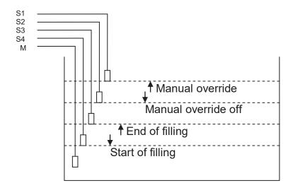
NIVA 5 uses 5 level probes. The probes must be positioned in the buffer tank so that the manual override level (S1) is below the buffer tank overflow.
