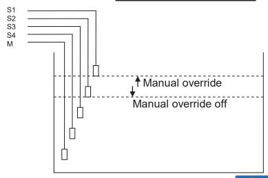
When the water level is high the overflow light lights up.
