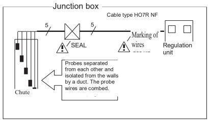
NIVA3) 1.5 mm <sup>2</sup> (HO7RNF type for example). To ensure a good performance of the installation, it is essential to ensure the sealing of the junction box and good galvanic insulation of the contacts. The use of silicone adhesive is recommended.
