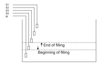
When the water level is low, the filling light lights up.
